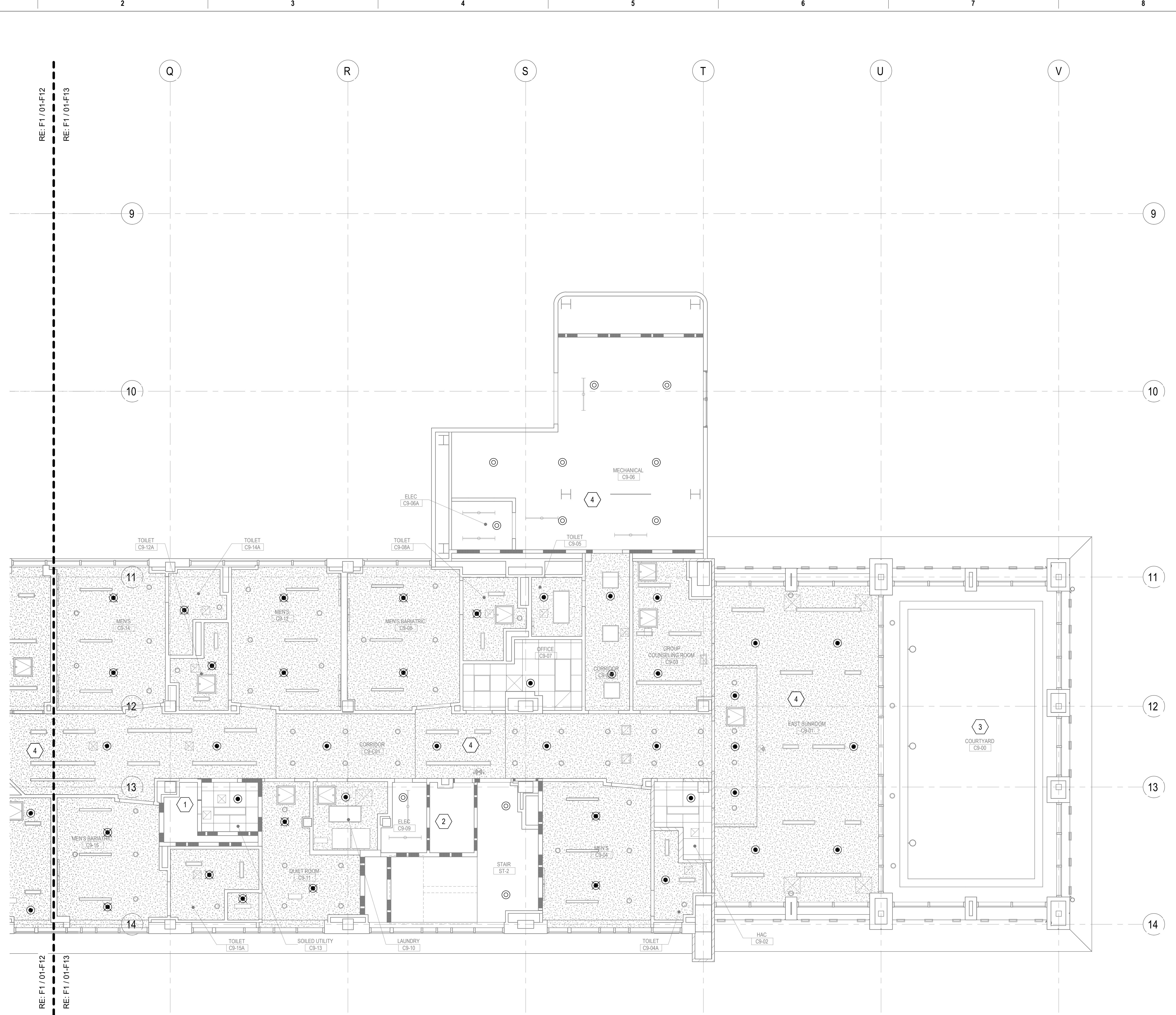
F1 9TH FLOOR FIRE PROTECTION PLAN - EAST 3/16" = 1'-0"
