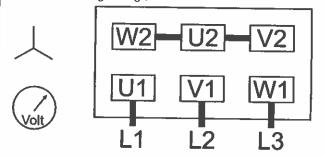
Double star connection, multi-voltage motor (low voltage):
