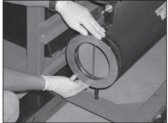
1B. Filter stop ring can slide between module header pipes after modules have slid together.
