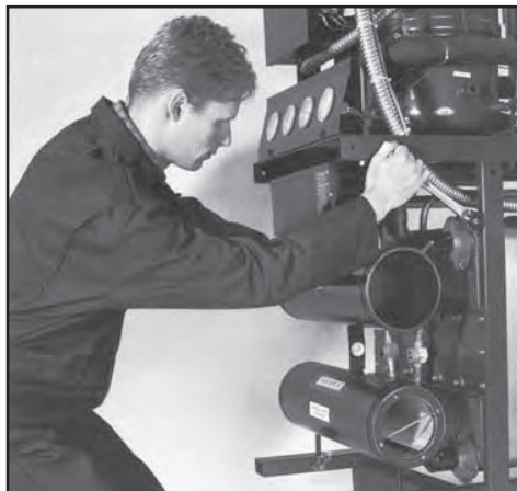
Figure 1, Removing header from heat exchanger.
