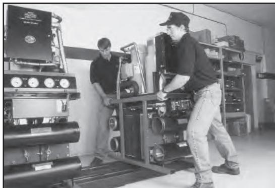
3. Place subsequent modules onto rails.
