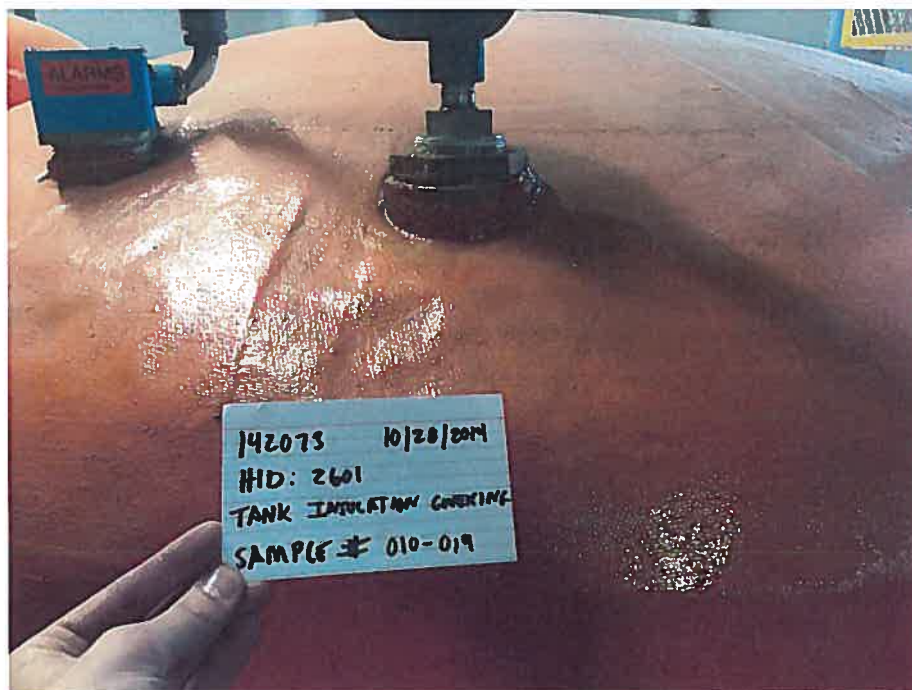
Figure 9: HID#2601 – Tank Insulation Covering Fiberglass
