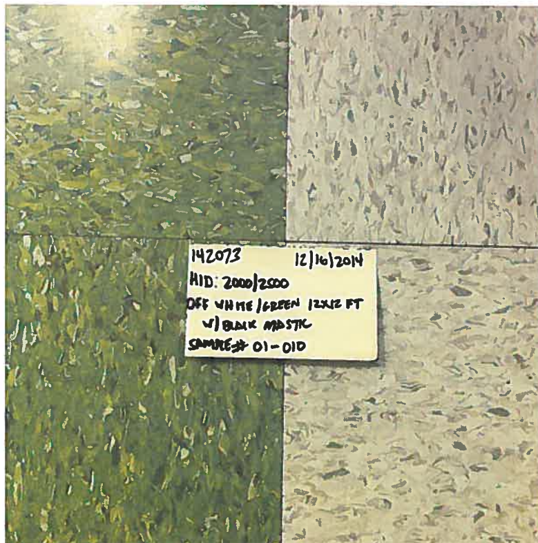
Figure 4: HID#2000/2500 – Off-White/Green 12"x12" Floor Tile (FT) w/ Black Mastic
